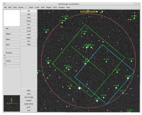
You can see the 5 stars inside the blue guide patrol field box. The number above each catalog star is the R-band magnitude. The R=14.000 magnitude star, which is star "7" in the table is a good guide star: not too bright or faint, and clear of the slit mask. Pick star #7:
