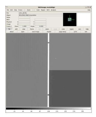
modsAlign will put up the interactive cursor on the ds9 display and ask you to mark the desired slit position for the target.
