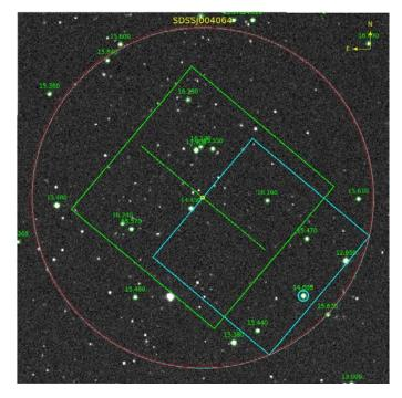
It indicates orientation (yellow N/E compass at the upper right), the relative scale, here shown by the 6-arcminute MODS science field of view (green box), labels the guide star (blue circle), and shows the slit and target positions.
