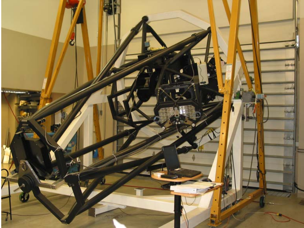
Figure 1. Photograph of the MODS1 instrument on its handling cart in the OSU Astronomy Department instrument assembly area. The photograph shows the entire MODS structure with all of the blue channel optics and mechanisms installed. The instrument is rotated on the axis of its handling cart, and as pictured is pointed about 20^\circ above the horizon.
