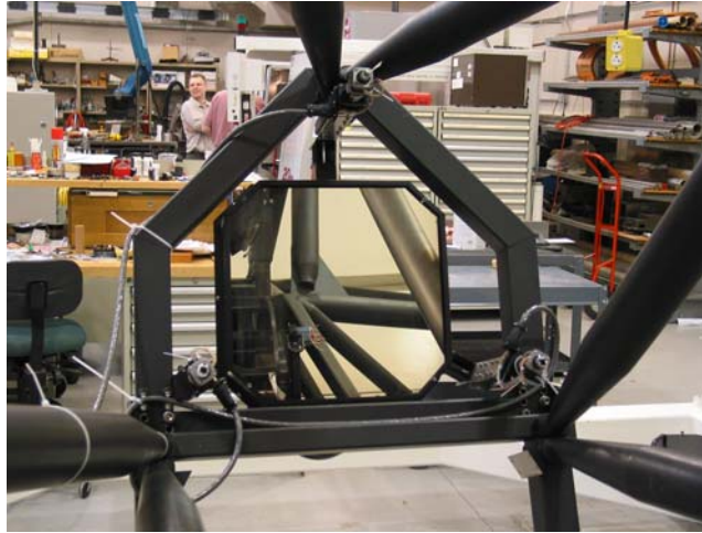
Figure 6 – MODS1 blue collimator assembly, showing the three tip/tilt/focus actuators and the collimator mirror. A temporary silver coating has been applied for alignment and IMCS testing activities.
