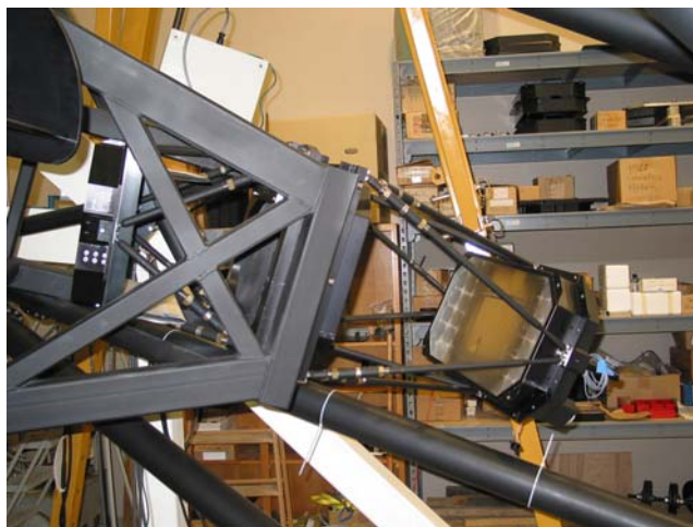
Figure 5 – MODS1 Blue Camera mounted for IMCS testing. Note the temporary silver coating in the center of the mirror. The camera is mounted without its filter wheel, CCD, corrector lens, or light-tight enclosure.
