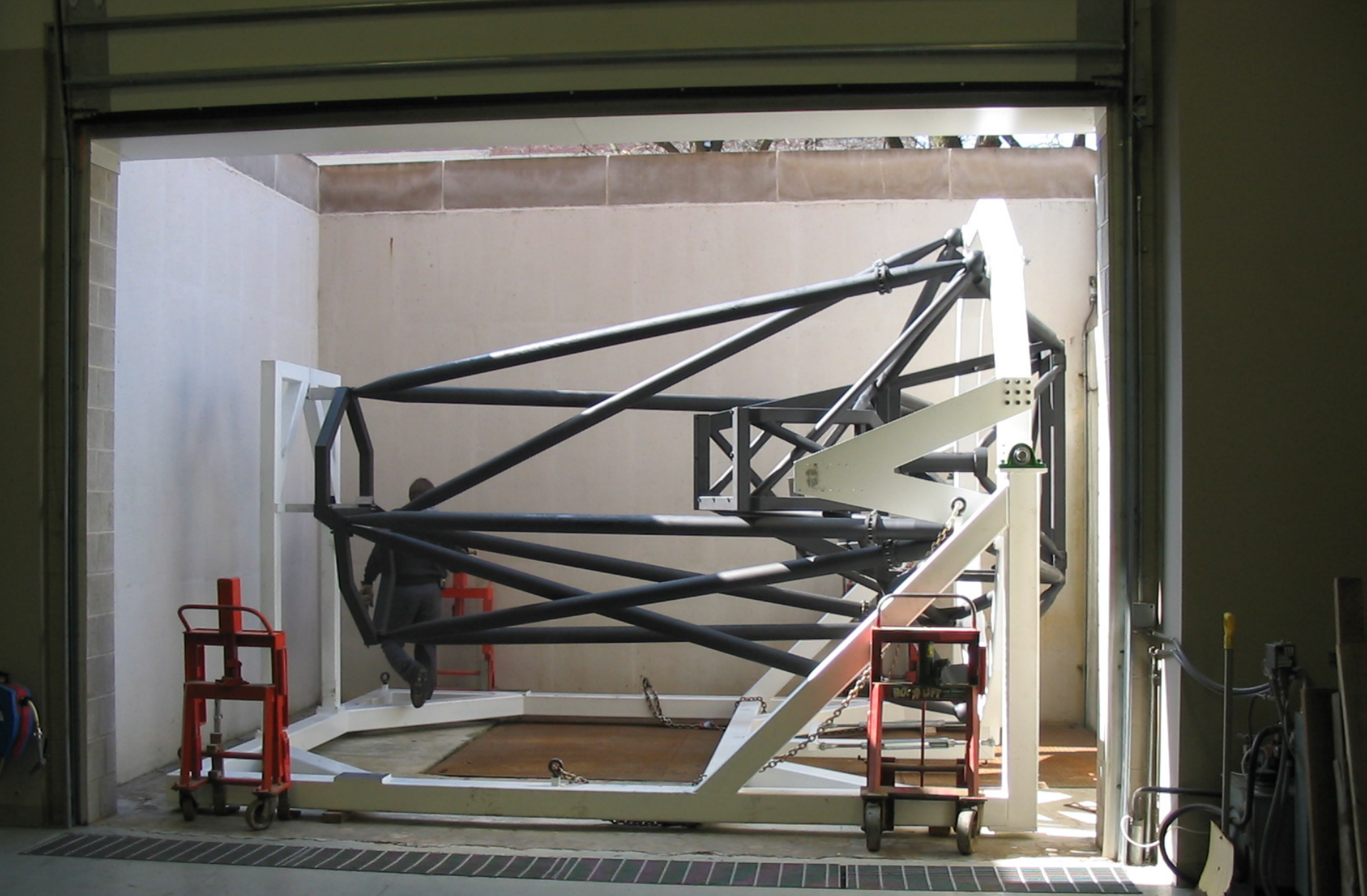
MODS Structure on Handling Cart
