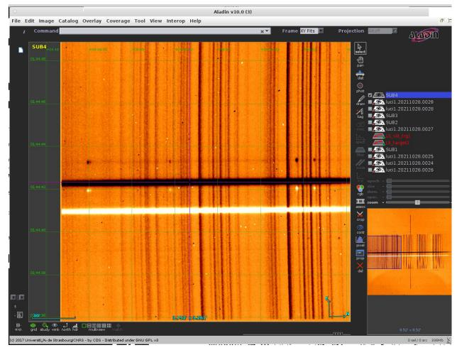
Observers Note: Emission lines are there. Dwarf is ~15" away from starlight still in slit. Dither is +/-10". Might have been better to do a larger dither, like 25"-30" to avoid negative in subtraction from affecting detection when pair subtracted and combined.
