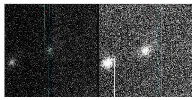
acquisition images: MODS1 on the left and MODS2 on the right. The green "+" marks the coordinate chosen as the center of the target and the red "+" marks the position on the slit to which it will be moved.
